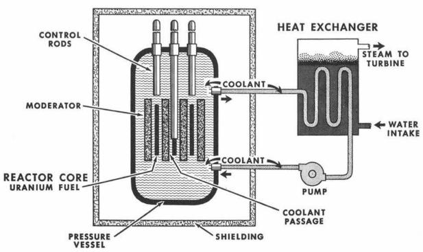
A REACTOR, basically, is an atomic furnace in which the fissioning or splitting of atoms of nuclear fuel can be controlled and put to useful work. The diagram shows the location of fuel, moderator, control rods, and coolant in a typical power reactor. These components are enclosed within a "pressure vessel" which
